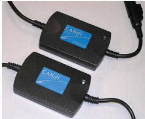
Can you tell the difference? The top CANdi module is counterfeit.
