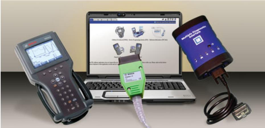
When to program or reflash an electronic control module is usually dictated by three conditions: directed by a technical service bulletin, installing a new control module, or a VIN search identifies a calibration update related to a customer concern.
